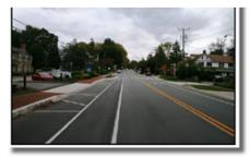
**Edge Line Striping**: Edge line striping is also effective in residential areas to narrow the lanes and/or provide additional delineation for other uses. Reducing the lane width has the potential for reducing speed by creating a narrower traffic lane. The area between the edge of the road and the lane marking can often be used for parking or as a bike lane, depending on the resulting shoulder width.
